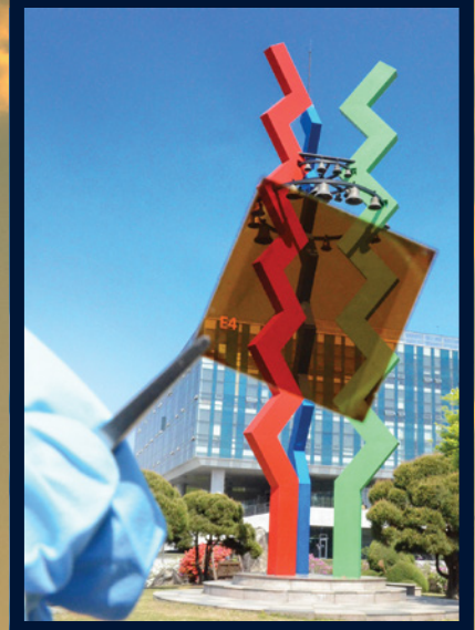
Prototype of a semi-transparent perovskite solar cell with thermal-mirror functionality
